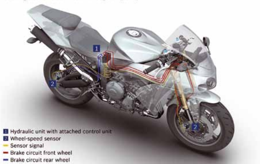
The components of Bosch motorcycle ABS including electronic Combined Brake System (eCBS)
